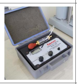
**Device: Resistivity Meter Model 88C** Function: Measure drilling fluid resistivity
