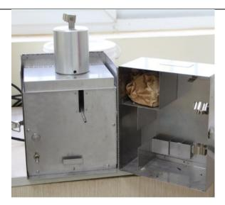
**Device: Retort 10ml Oil and Water Kit Model 871**Function: determine the quantity of liquids and solids in a drilling fluid
