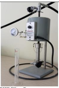
**Device: HPHT Filter Presses** Function: Evaluating the filtration properties of drilling mud at high temperatures
