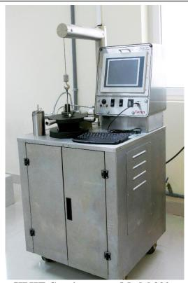
**Device: HPHT Consistometer Model 290**Function: Measure cement slurry viscosity or consistency under elevated
