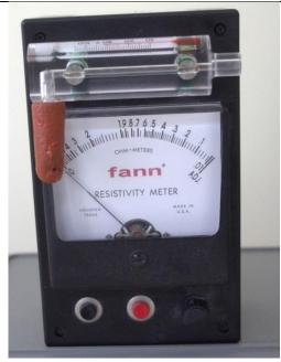
**Device:** Model 653B Resistivity Meter Function: Measure the resistivity of fluids
