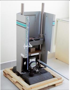
**Device: Compressive Strength Tester**Function: measuring the maximum amount of compressive load a material can bear before fracturing
