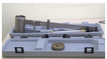
**Device: Balance Density TruWate Model 141** Function: Measuring the absolute density of a fluid sample
